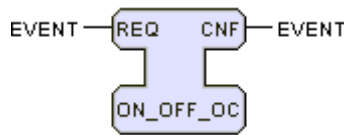
Figure 2.5 Composite Function Block with Input and Output Events
