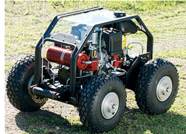
The $3995 Parallax Propeller QuadRover robot is controlled by the multicore Propeller chip.
