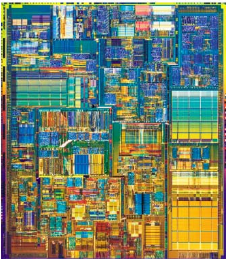
2000: Intel Pentium 4 Processor Clock speed: 1.5 GHz # Transistors: 42 million Technology: 0.18 \mu m CMOS
