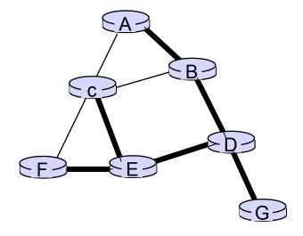
(b) constructed spanning tree
