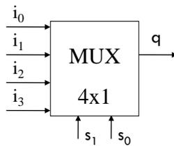
$$f(i_3, i_2, i_1, i_0, s_1, s_0) = i_3 s_1 s_0 + i_2 s_1 s_0' + i_1 s_1' s_0 + i_0 s_1' s_0'$$
